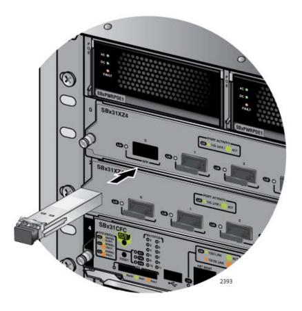
Figure 105. Installing an XFP Transceiver in the AT-SBx31XZ4 Line Card
